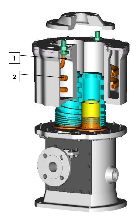
Indirect cooling of the working chamber:
