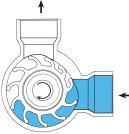
The rotating impeller carries the liquid from the inlet towards the outlet port. During this part of the cycle, the volume between the wings remains virtually constant. The distance between the wings allows
