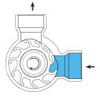
Due to the eccentric interior cross-section of the pump body, a partial vacuum is created as the volume increases between the flexible impeller wings at the inlet port. The resulting suction draws the liquid into the pump.
