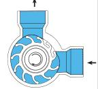
The liquid is discharged from the pump in a continuous, uniform flow when the wings bend, thus decreasing the volume between them, as they come into contact with the flattened part of the
