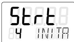
The positioner runs through several initialization steps during the automatic initialization process. The lower line of the display indicates which initialization step is currently being run through. The initialization process depends on the actuator used, and takes up to 15 minutes.
