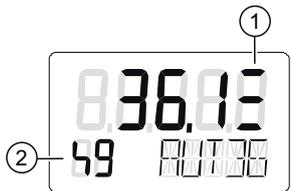
Figure 8-8 Display of a threshold 3 error message with three columns (maintenance alarm)
