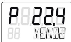
9. Confirm with the
