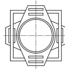
**Type Lateral expansion joints as Double Hinge Unit PN 10 – PN 25, multi-ply from DN 40**
