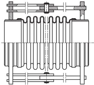
**Type Angular expansion joints, movable on all sides PN 10 - PN 25, multi-ply from DN 40**
