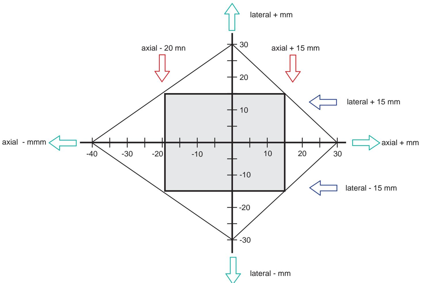
The current movements in combination must fit into the movement diamond as a rectangle.
