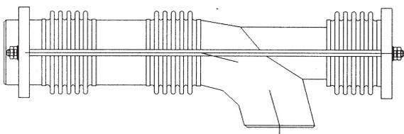
**Type Heating compensator DN 15 - DN 50**
