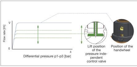
The pressure independent control valve "Cocon QTR/QFC" is a valve combination consisting of an automatic flow regulator (with manual nominal value setting) and a regulating valve. The pressure independent control valve can be equipped with an
