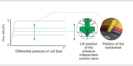
The pressure independent control valve "Cocon QTZ" with automatic flow control is a compact valve combination consisting of a flow regulator and a regulating valve. The nominal value of the flow regulator can be set with the help of an easily accessible handhweel.
