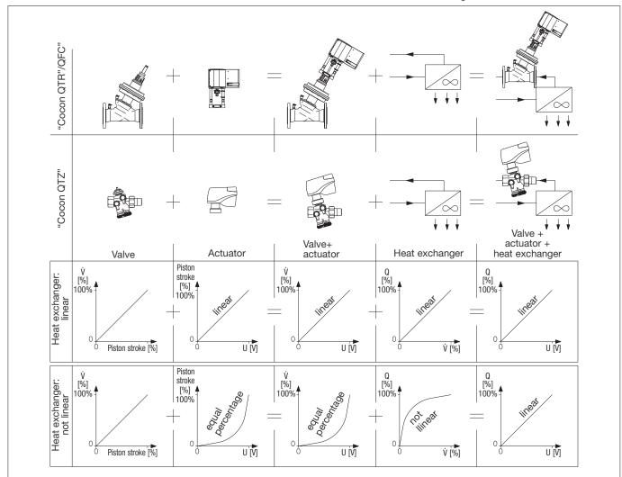
Optimisation of the interplay of valve, actuator and heat exchanger with modulating 0-10 V actuators.
