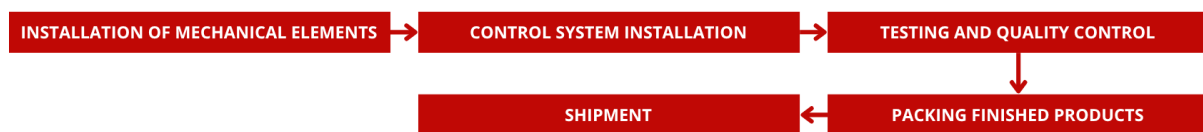
Figure 5.2: Diagram of the production process of GuardPro air curtains
