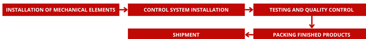
Figure 5.2: Diagram of the production process of Guard air curtains
