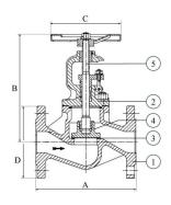
Stellite-reinforced sealing between seat and globe.
