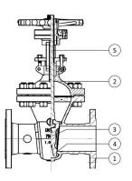
Stellite-reinforced sealing between seat and wedge.
