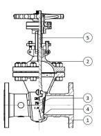
Stellite-reinforced sealing between seat and wedge.
