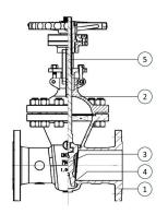
Stellite-reinforced sealing between seat and wedge.
