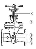
Stellite-reinforced sealing between seat and wedge.
