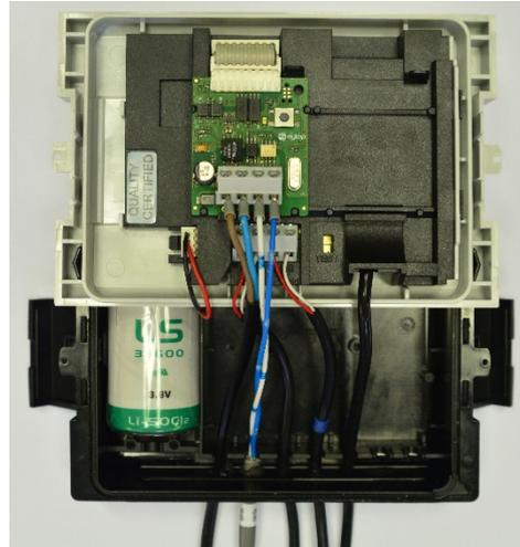
Picture 5.6 - Example of correctly wired module
