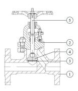
Stellite-reinforced sealing between seat and globe.
