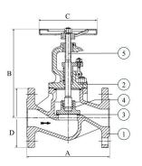
Stellite-reinforced sealing between seat and globe.
