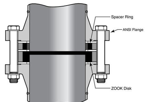
When replacing a metal rupture disk with a ZOOK Graphite Rupture Disk, a graphite lined armored spacer ring can be provided to fill the space of existing flange face-to-face distance, eliminating the need for piping modifications.
