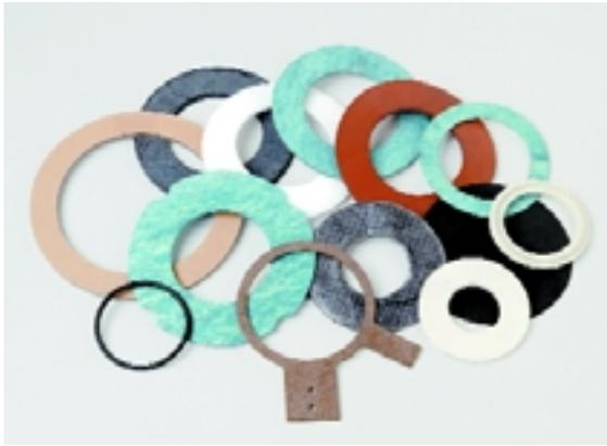
Gaskets used with graphite disks are stocked in the following materials: Neoprene, Non-asbestos, solid PTFE, and PTFE envelope. Gaskets can be supplied loose or attached to the disk (Note: field replacement of gaskets NOT recommended on TWO-WAY Disks or Insulated Units)
